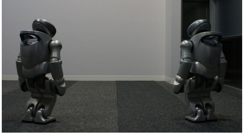
Figure 7.3: Calibration phase of the vision system. Both robots are shown an empty environment for some extended period of time, allowing them to observe the statistical characteristics of the scene background.
