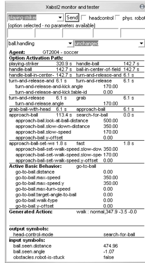
Fig. 4. An example for a XABSL monitoring tool using the debugging interfaces of the XabslEngine (inside the GermanTeam’s RobotControl application).
